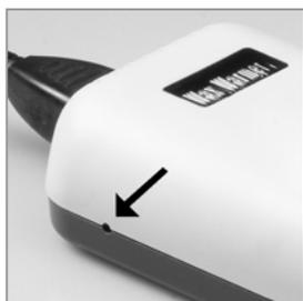
On the left side of the unit, it is possible to insert a small screwdriver to activate an adjustable trimmer. When the device is totally turned to the minimum (leftwards) the sensibility is low (longer detection time); when turning it rightwards, sensibility will be increased. It is recommended to set the device in the middle position of the scale.
