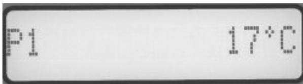
P1 or P2 on the left part of the display indicate the last modified program. On the right side, the internal temperature is shown.
