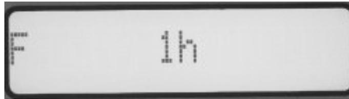
The **F** parameter is the additional time for temperature holding at the end of the cycle. This is an extra time to allow burning in case of more rings, or should the operator neither be present nor ready. Their value is expressed in hours, minimum is 1 hour. By pressing ENTER the user goes back to STAND-BY screen.
