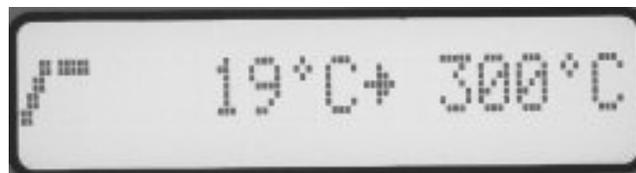
The lines on the left part represent the burning cycle graph: during raise in temperature, the curved portion will blink; on the right part of the display the target temperature is shown; in the middle, the detected temperature is shown. During stabilization stages, the horizontal portion of the graph will blink. In the middle of the display, the remaining time will be shown, while on the right side the actual temperature is displayed.
