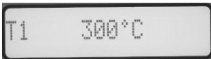
Set by ▲ and ▼ the temperature **T1** of the first stage, then confirm by ENTER
