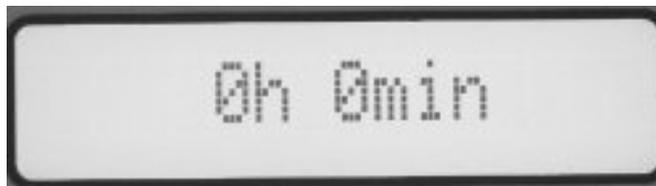
At this stage, **scheduled delayed time (in hours and minutes) can be inserted**. To start immediately, confirm by ENTER the 0 value. To schedule a switch-on time, insert by means of the arrows both parameters and confirm by ENTER. The display shows a countdown to cycle start, when this will be 0 the furnace will start.
