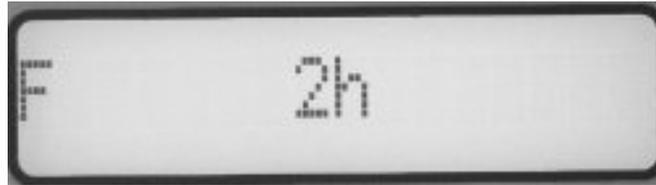
Set the temperature holding time for the final temperature (during this time, sub-cycles specific for any casting ring can be set), then confirm by ENTER and return to STAND-BY screen.
