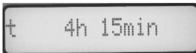
Set temperature holding time **t**: set hours, confirm by ENTER set minutes, confirm by ENTER
