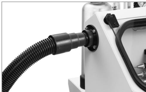
Any other suction system can be connected to the black collection intake by means of flexible piping; the inside manifold fits a  $\varnothing$  30mm pipe, the outside manifold fits a  $\varnothing$  40mm pipe.
