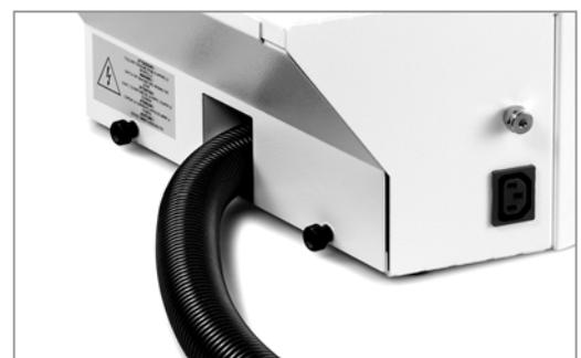
5. Adjust the air flow to avoid the machine being under pressure. Slightly turn the mobile section of the adjusting valve when the suction system is on and stop when you notice that the gloves are still slightly inflated.
