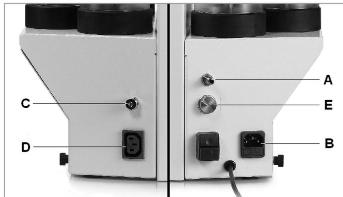
2. Insert the quick clutch fitting on the male intake (A) located on the right side of the unit and connect the pneumatic feeding pipe (polyethylene or rilsan, with diameter  $\varnothing$  8x6) to the pipe-fitting. It is also possible to use a  $\varnothing$  12x6 elastic feeding pipe, by using the fitting supplied with the unit.
