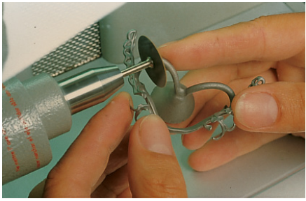
Disconnecting the sprues
