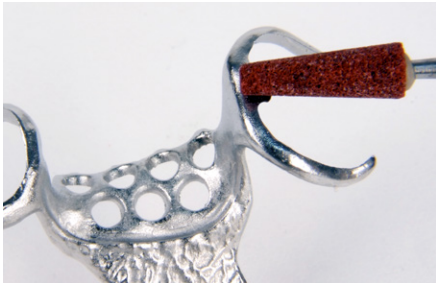
Finishing with corundum or fine grinding stones
