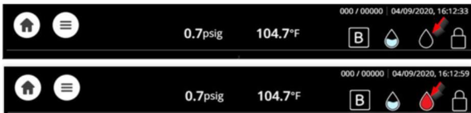
The following screen shows that the Waste water tank is full.
