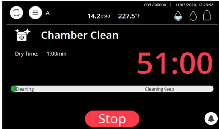
17. After 45 minutes the chamber clean process is completed, the chamber is clean, and the following screen is displayed.
