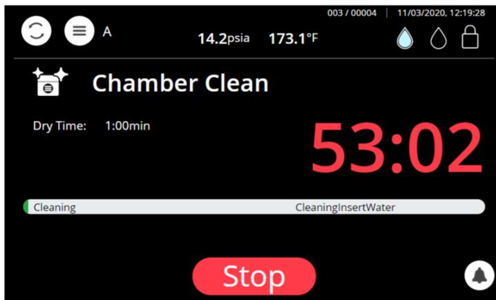
The warming up to 176°F and hold for 10 minutes at 176°F, (This stage uses 500ml of water from the clean water reservoir). Exhaust water from the chamber, goes to air removal, pass to plateau of 3 minutes at 269.6°F and 1 minute drying time.
