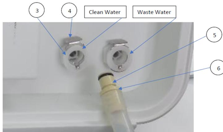
2. Put the other end of the hose into a drain bucket.
