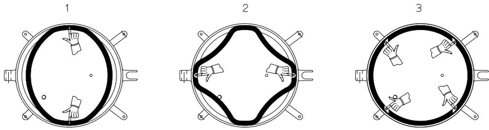
Pull off the gasket from the door groove. Install the new gasket as described in drawings 1, 2 and 3 above.
