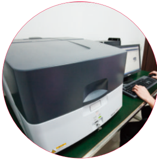
Energy dispersive X-ray fluorescence spectrometer To decter the harmful materials, according to the demand of EU standard
