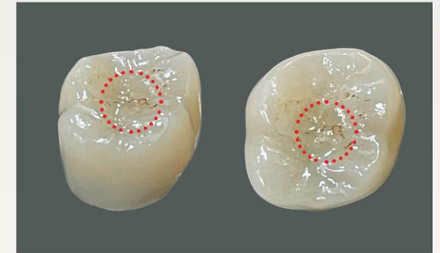
Test result from Chewing simulator proves superior wear-out resistance in occlusal region.
