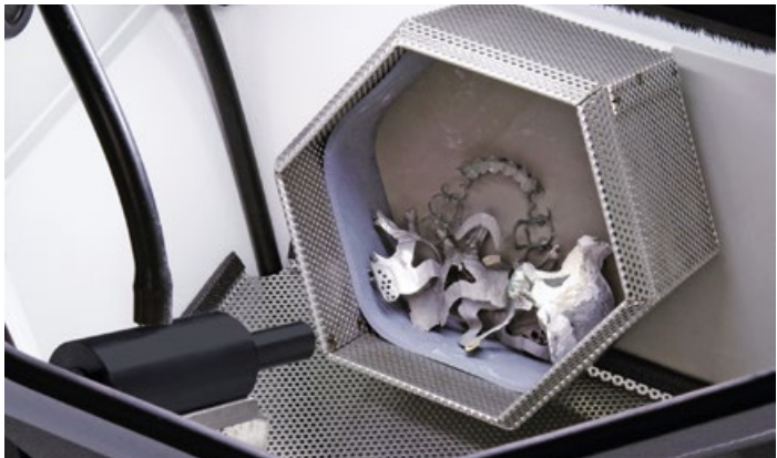
Saves time and money: the large rotating steel basket allows up to 7 objects to be sandblasted at the same time
