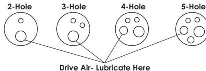
**Weekly:** Place a few drops of lubricant in the swivel junction in the middle of the handpiece and twist swivel to work lubricant into junction and wipe clean.
