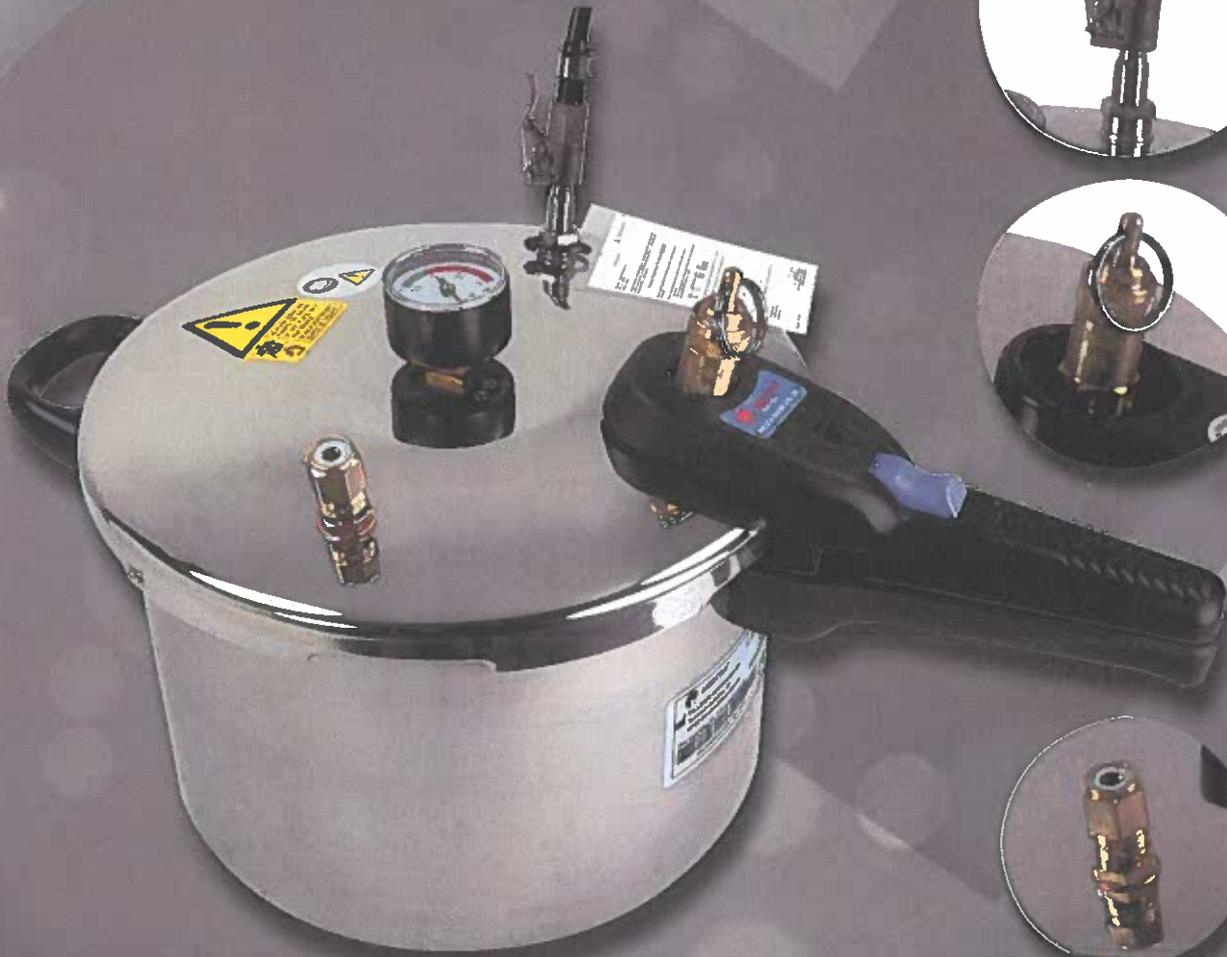
For cold and hot polymerizing at pressures up to 2 bar.
