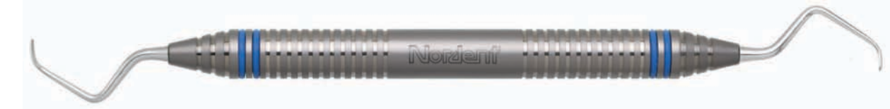
Rigid Gracey #9-10 Long contra-angle for molars and less accessible root surfaces. Terminal shank reach is 12 mm.
