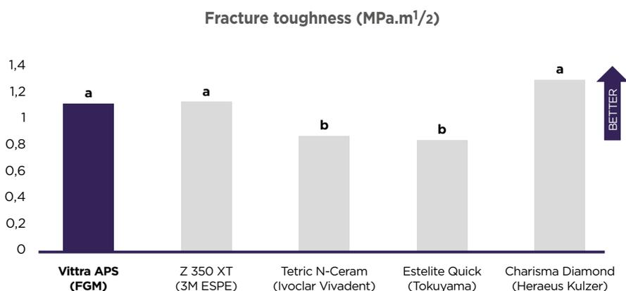
**Figure 4: Fracture toughness (mean and standard deviation in MPa. m<sup>1/2</sup>) of different composites (n=10) (1-way ANOVA and Tukey test; p<0.05).**
