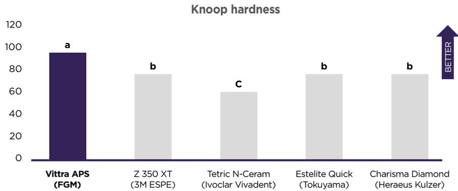
**Figure 5: Knoop hardness (mean and standard deviation in KHN) of different composites (n=5) (1-way ANOVA and Tukey test; p<0.05).**
