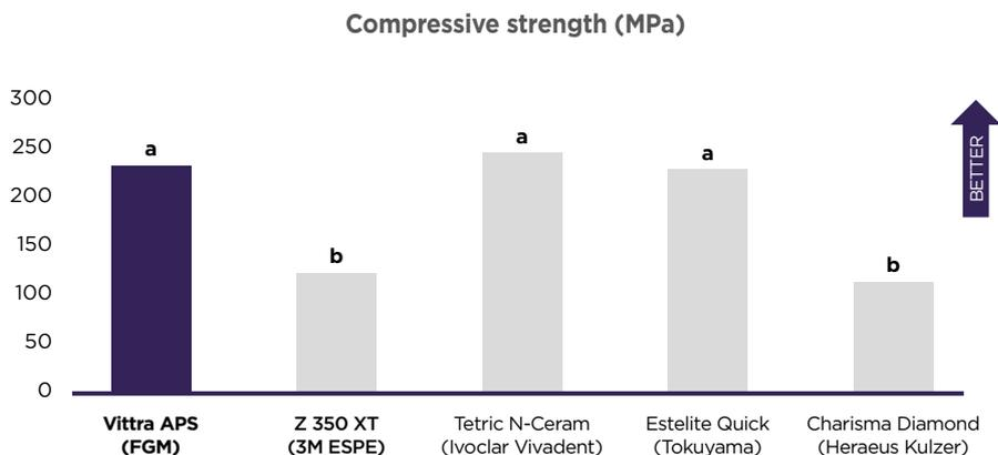
**Figure 3: Compressive strength (mean and standard deviation in MPa) of different composites (n=10) (1-way ANOVA and Tukey test; p<0.05).**
