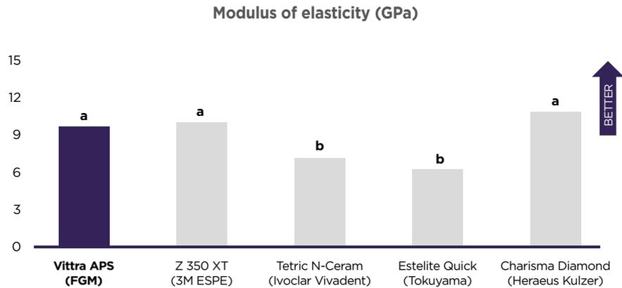
**Figure 2: Modulus of elasticity (mean and standard deviation in GPa) of different composites (n=10) (1-way ANOVA and Tukey test; p<0.05).**
