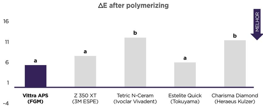
**Figure 8: Shade variation (mean,  $\Delta E$ ) before and immediately after polymerization (n=3) (1-way ANOVA and Tukey's test;  $p < 0.05$ ).**
