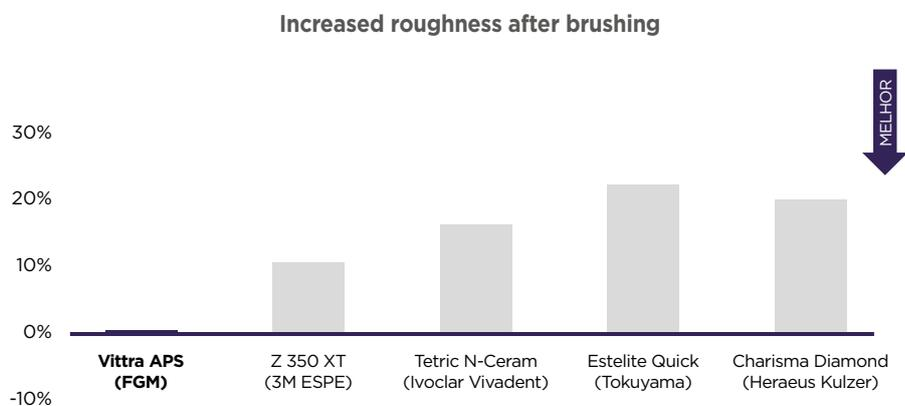
**Figure 7: Roughness increase (mean in %) after simulated brushing (n=10).**
