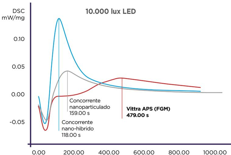
**Figure 9: Working time (average in seconds) of the Vittra APS composite and two other composites: one nano-hybrid and one nanoparticulated.**
