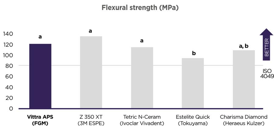
**Figure 1: Three-point flexural strength (mean and standard deviation in MPa) of different composites (n=10) (1-way ANOVA and Tukey test; p<0.05).**
