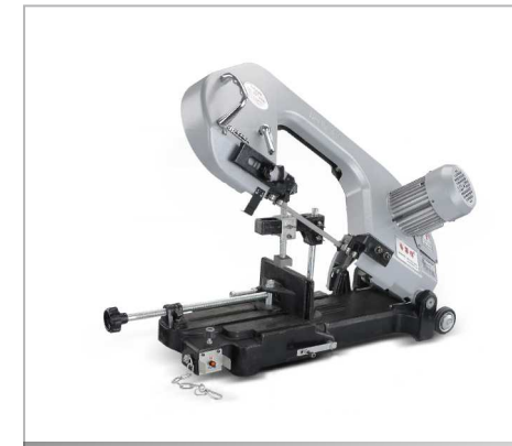
小锯床 The cutter for cutting the metal crown
