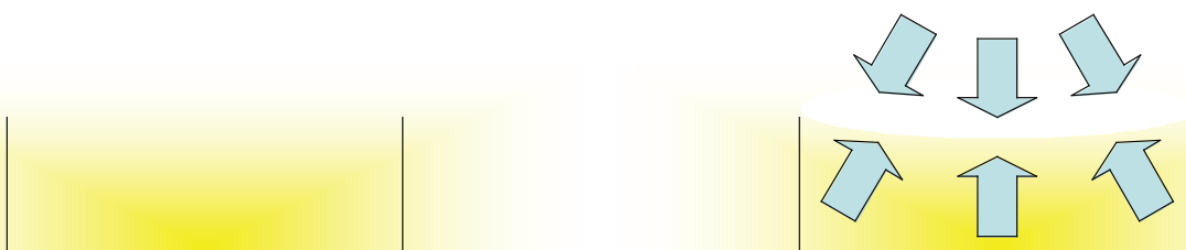
Figure 7b. Composites with a high modulus of elasticity. These can only deform slightly during polymerization. Shrinkage stress will occur at the free surface and at the composite/tooth interface.
