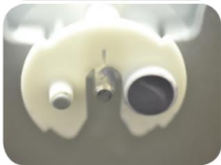
Make sure to have no excess materials at the end of the cartridge.
