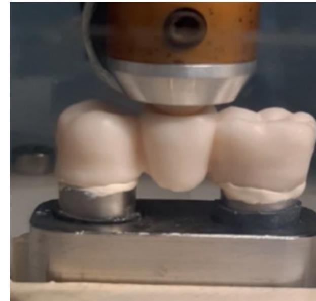
Figure 2: Test setup in the chewing simulator
