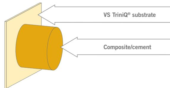
Figure 10: Setup of the shear bond test
