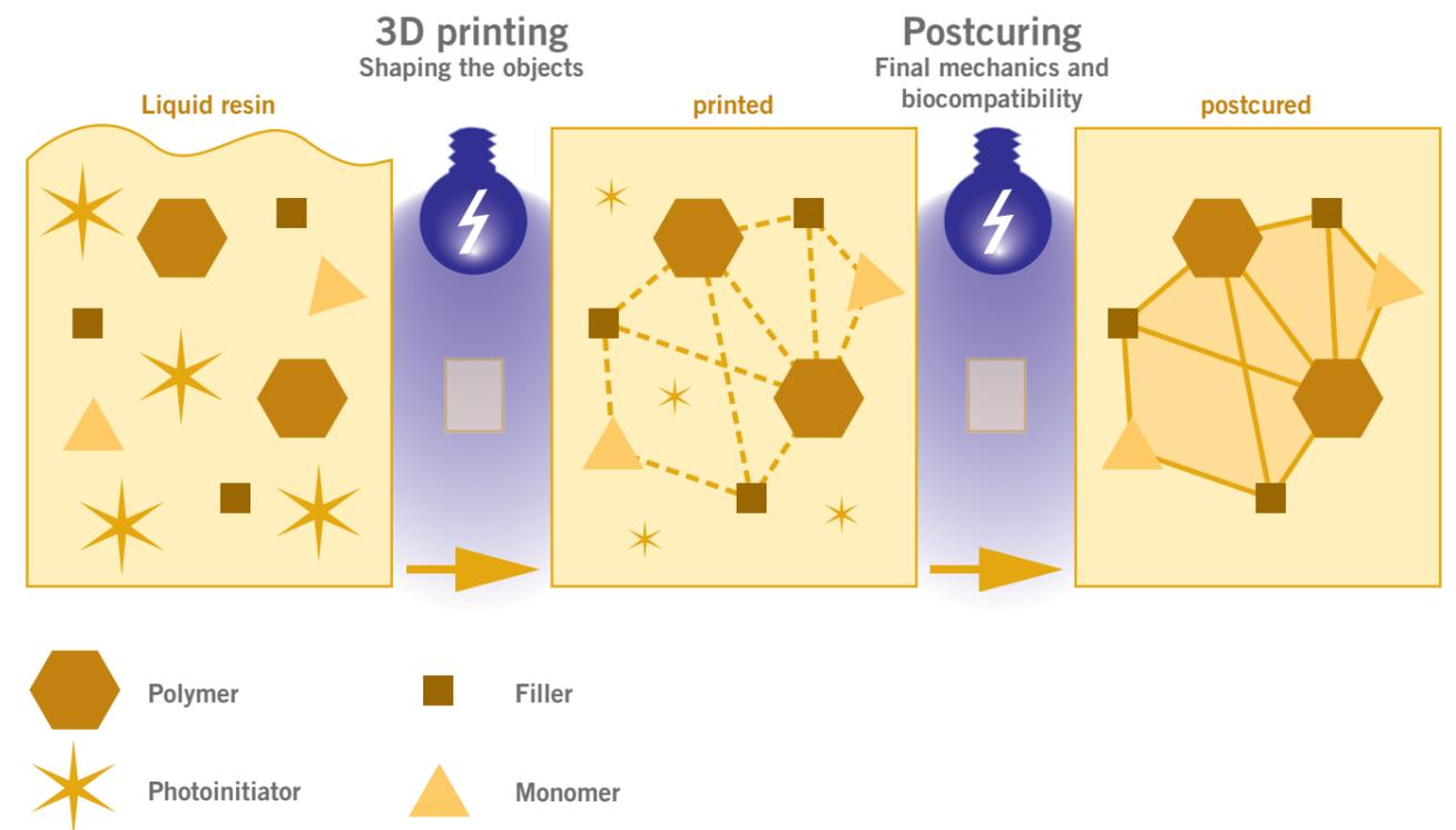
Figure 11: Polymerization during the 3D printing workflow
