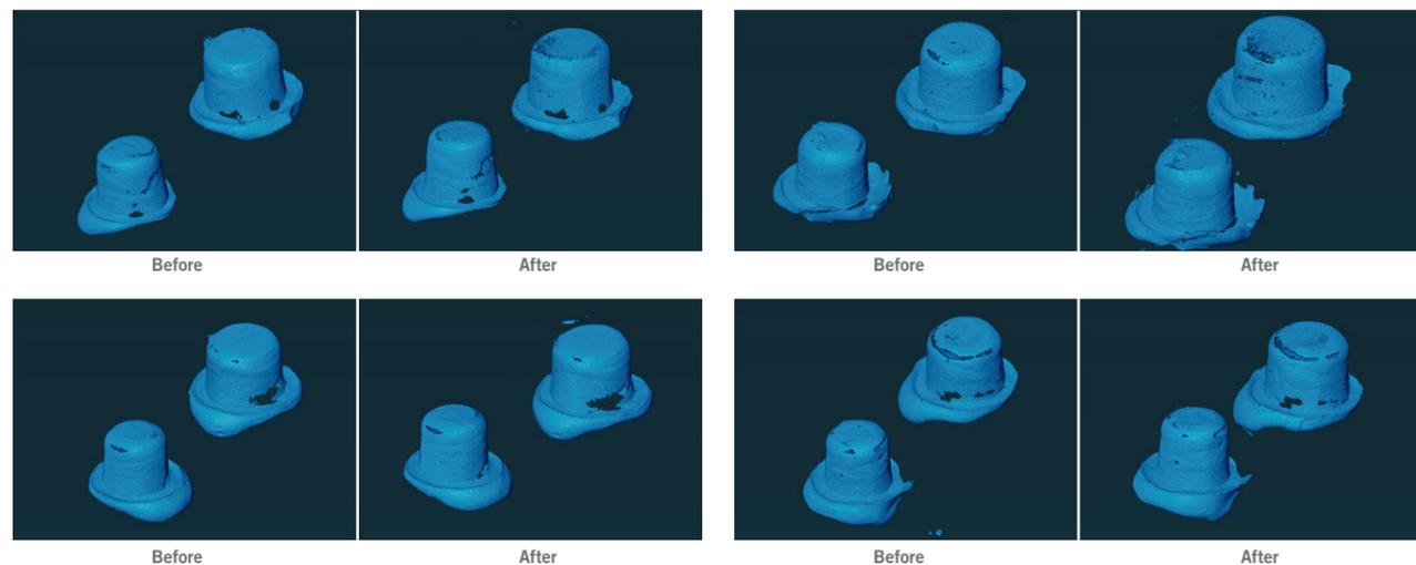
Figure 4: Examples from the µCT analysis (4 of 16) before and after 10-year chewing simulation
