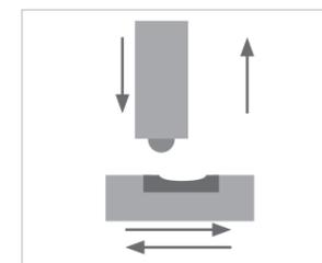
Figure 8: Schematic diagram of the POB chewing simulator
