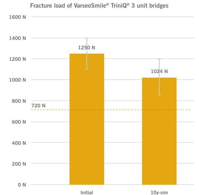
Figure 3: Mean breaking loads for the baseline and the artificially aged test group of three-unit bridges made of VarseoSmile® TriniQ®
