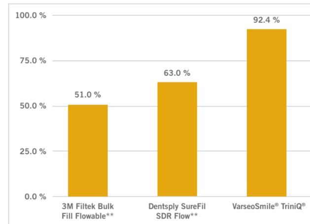
Figure 13: Conversion rate of the double bonds
