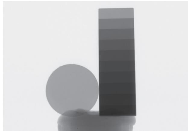
Figure 7: VarseoSmile® TriniQ® specimen next to an aluminum step wedge
