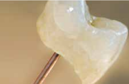
Cracks in the ceramic
