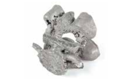
Rough casting due to overheating
