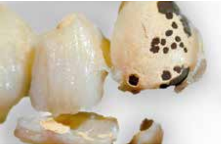
Bubbles in opaquer due to casting errors or incomplete evaporation of glycerine
