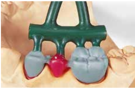
4 mm wax wire for feeding from the base socket mould former to the distribution channel
