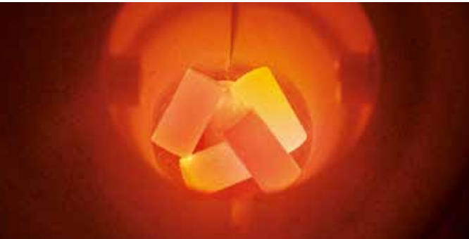
Preheating the alloy in Nautilus®
