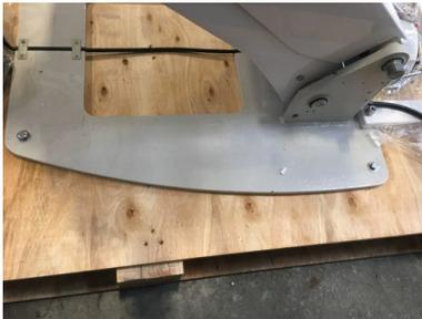
3. Remove the lift handles from the pallet. Install on the threaded hub on each side of the chair. These are going to be used as a lift point. **Do-not use the chair armrest as lift points.**
