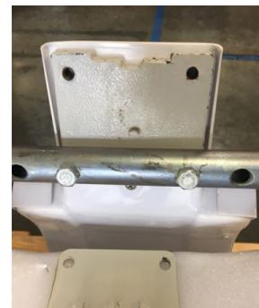
4. After the chair is placed in the installation location, Install the leveling lugs included in (bag B) in the holes that were used to secure the chair to the pallet. These will be used to level the chair base in the event the floor is not level.
