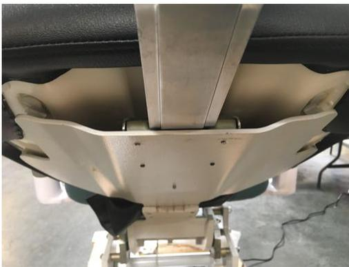
3. Place the backrest cover over the backrest bracket. Secure in place using the 4 Allen screws and washers in Bag (D). TIP: You can use an Allen wrench to align the lower holes, so the Allen goes in straight. Once all 4 Allen screws are installed, tighten them to secure the cover in place.
