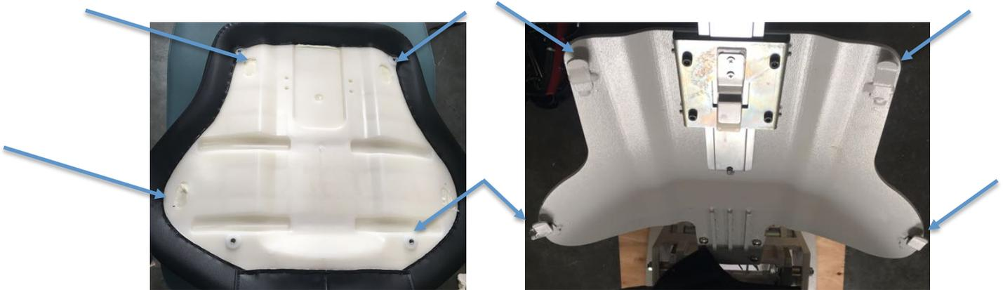
2. Once all 4 tabs are aligned with the backrest cushion slots, Slide the backrest down to secure in place. Verify all 4 corners are secured.
