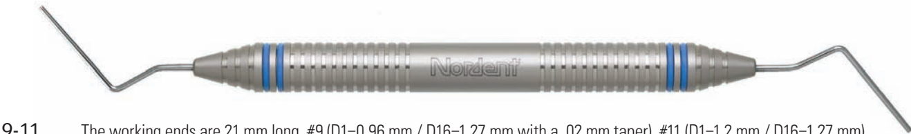
9-11 The working ends are 21 mm long. #9 (D1=0.96 mm / D16=1.27 mm with a .02 mm taper) #11 (D1=1.2 mm / D16=1.27 mm).
