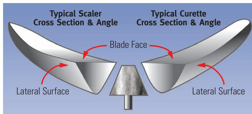
With InstRenew you focus on sharpening the blades and forget about positioning the shanks. Every Brand and Every Pattern of Scalers and Curettes have one thing in common. The angle between the blade face and the lateral surface, that creates the sharp edge, is always the same.
