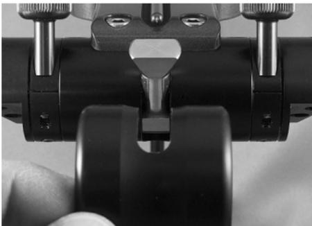
cover which aligns with the centric latch lever and allows it to travel freely. Grip the upper member firmly with one hand. Holding the dust cover with the other hand, align the slot with the latch lever and firmly push the cover onto the pivot bar.
