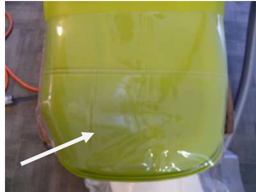
Figure 83: Install the foot protector at the end of the seat.
