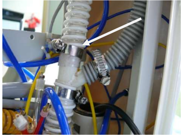
Figure 36: Attach the drain tube to the 'Y' connector. Use a hose clamp to secure it.
