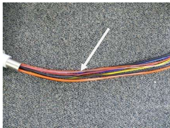
Figure 52: Straighten and untangle the tubes and cables at the end of the flex arm.
