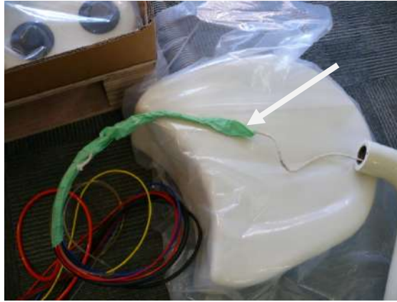
Figure 54: Use masking or electrical tape to attach the tube/cable bundle to the rope in the 'S' pipe. Carefully push and pull the bundle through the 'S' pipe narrow end.
