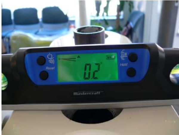
Figure 18: Use a level in both directions and tighten the setscrews in the post hole.
