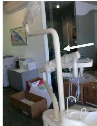
Figure 70: Pass the cable down the straight pipe and insert the 'S' pipe into the straight pipe.
