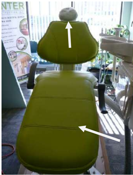
Figure 82: Insert the headrest into the top of the backrest. Install the seat. There are 4 bolts that hold it to the chair frame.
