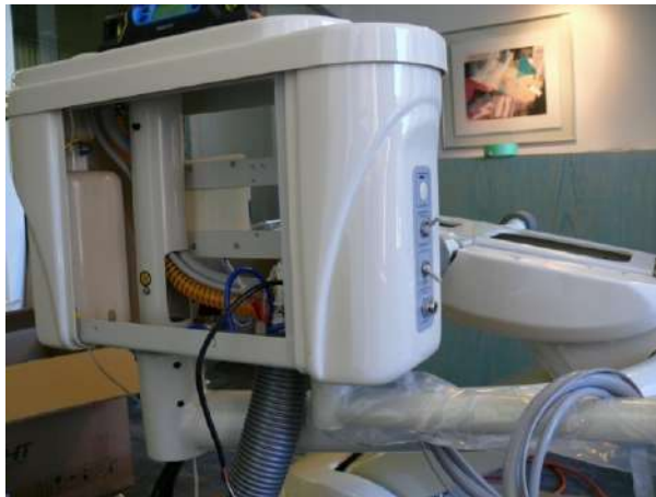
Figure 18: Use a level in both directions and tighten the setscrews in the post hole.
