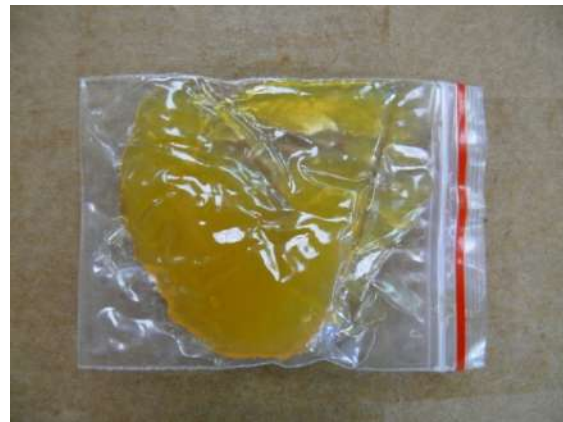
Figure 43: Bag of grease. Use this to grease all the bare metal parts.
