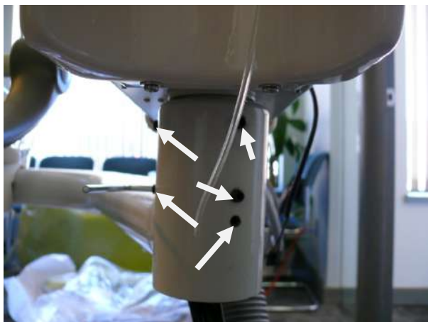
Figure 17: Use these setscrews to hold and level the side box. The lowest one supports the bottom of the pipe. There are 6 other setscrews to adjust the side to side level. The box should be parallel to the chair.
