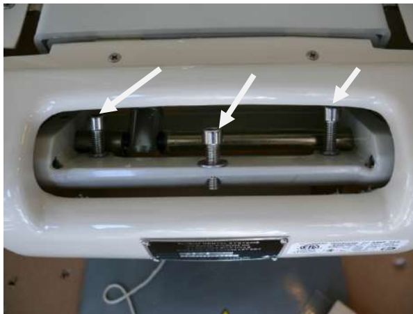
Figure 79: Attach the backrest to the chair. See the 3 bolts in the backrest assembly. Use the foot control to move the backrest to a position where the bolts can be accessed.
