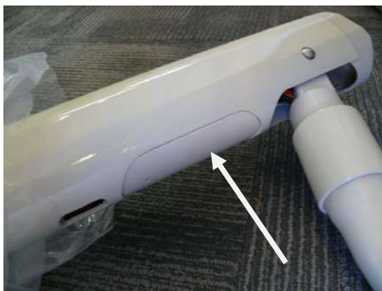
Figure 51: Pull any slack tubes and cables out to the end of the flex arm. The light blue tube is just folded over and inserted into the arm. Avoid kinking it. Re-install the plastic oval cover.
