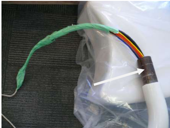
Figure 55: Pull all the slack from the tubes/cables. Connect the 'S' pipe to the arm. Grease the bare end.
