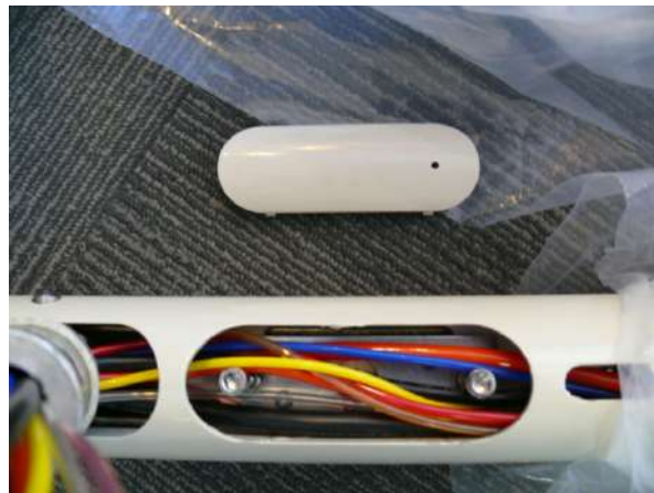
Figure 45: Remove the oval cover. Use an Allen wrench in the cover hole to pull the cover off.
