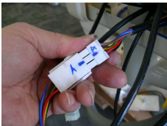
Figure 61: Connect cables by matching the labels.
