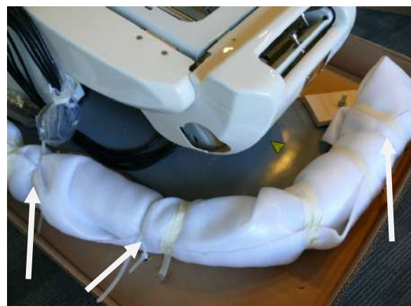
Figure 6: Cut the nylon ties holding the chair bracket to the pallet. Unwrap the chair bracket.
