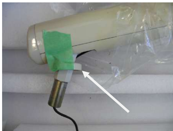
Figure 64: Install the small plastic ring as shown. Grease the bare metal parts.
