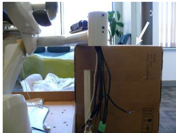
Figure 12: Use a box to support the bracket. Either use the string or simply push them through one at a time, starting with the biggest connector. Avoid kinks.
