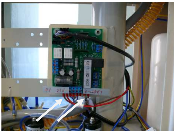
Figure 27: Connect the wires for the light to the circuit board. They are labeled 0V, 24V, and K-Light. The board will also have labels.
