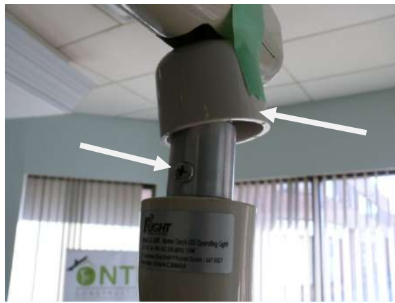
Figure 74: Insert the arm end into the lamp head and attach with the screw removed earlier. Drop the plastic cover down.
