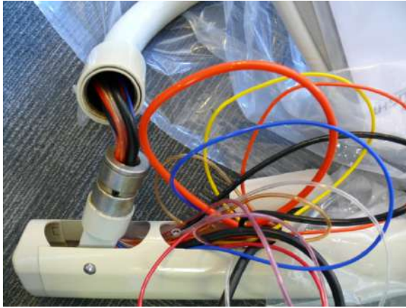
Figure 46: Carefully push and pull the tubes and cables from the treatment tray and out the oval opening. Grease the bare metal.
