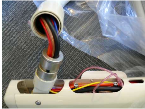
Figure 47: Pull the same tubes and cables from the end of the flex arm to take up all the slack at the oval opening. This will move the parts together.
