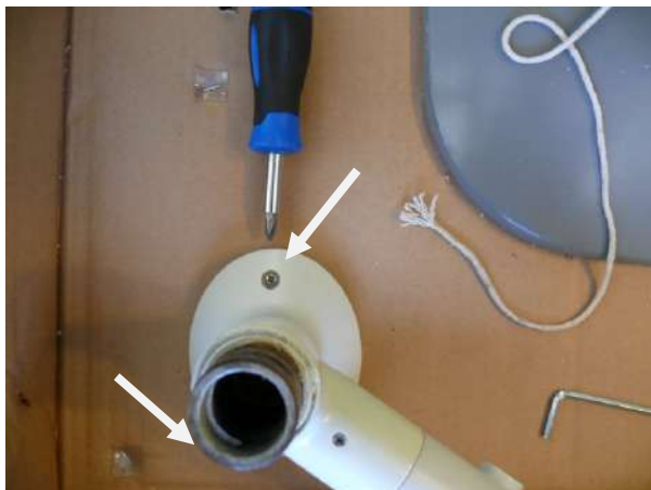
Figure 21: Remove the 2 screws holding the assistant touchpad. Install the HP holder to the assistant post. Push the cable through for the touchpad.
