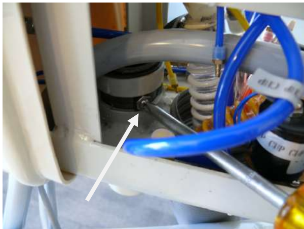
Figure 39: Install the nut and screw in the assistant arm. They are in a bag in the side box. A screw holder is helpful to get it started.
