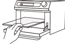
Place the glass panel inside the curing chamber before use
